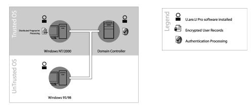
However, if the sensor is connected to an NT workstation that is part of a trusted NT domain, then that local workstation sets up the challenge/response link with the sensor and performs feature extraction on behalf of the authentication server.
